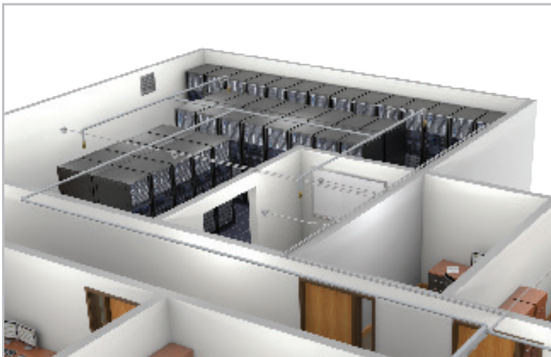
725 psi systems make it possible to locate agent supply away from the protected area.
